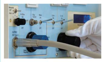
Q-unit is equipped with useful functions for different test, inspection, and maintenance works: on-off controls for driving air, cooling water, chip air, and illumination. In addition, Q-unit has an air-blow system to discharge cooling water remaining inside of the handpiece after use.
