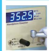
Q-unit has two sensors to measure number of revolution and frequency.
